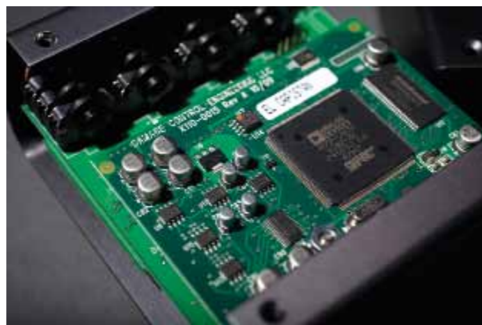
A powerful SHARC DSP chip is at the heart of these analogue-emulating pedals
